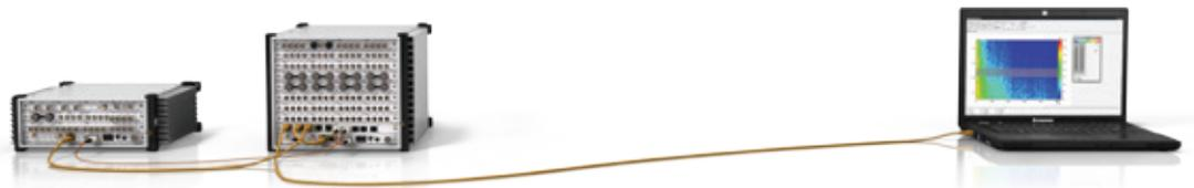
More than 4 Mainframes can also be synchronized. This requires additional Synchronization Engines which can also be housed in one of the Mainframes. Limitless Mainframes can be synchronized for an unlimited channel count, greater geographical reach and an efficient use of available hardware.
