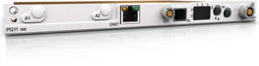
The PQ11 G2 is a dual function board combining a VMEbus System Controller, Master, Arbiter and Interrupt Handler with VMEbus Power Supply. It can be used in an MF02 and MF03 Mainframe. It is an entry level board particularly suited to smaller Mainframes.
