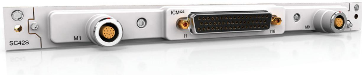
Four high speed ICP® based Modules are integrated with an SC42S Signal Conditioning board to provide a single Compound-Module, the ICM42S. This provides 16 ICP® or voltage input mode channels as well as 16 monitoring output channels.
