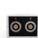
Provides 2 sets of 4-way Lemo EGG.0B connectors for use with 2 Pt100 sensors. These connectors provide current to a Pt100 sensor and sense the voltage across it.
